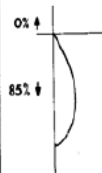
R-40 flood with specular anodized reflector skirt; 45° cutoff
