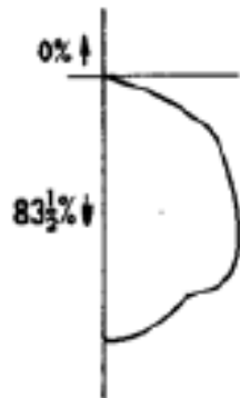
Porcelain-enameled ventilated standard dome with incandescent lamp
